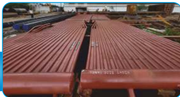
Boiler Panel final inspection
