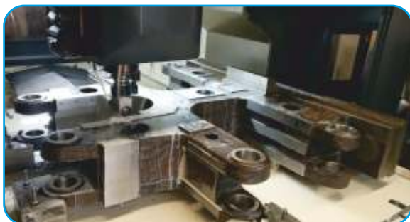
Sugar Mill Machining Precision- 0.010-0.015mm
